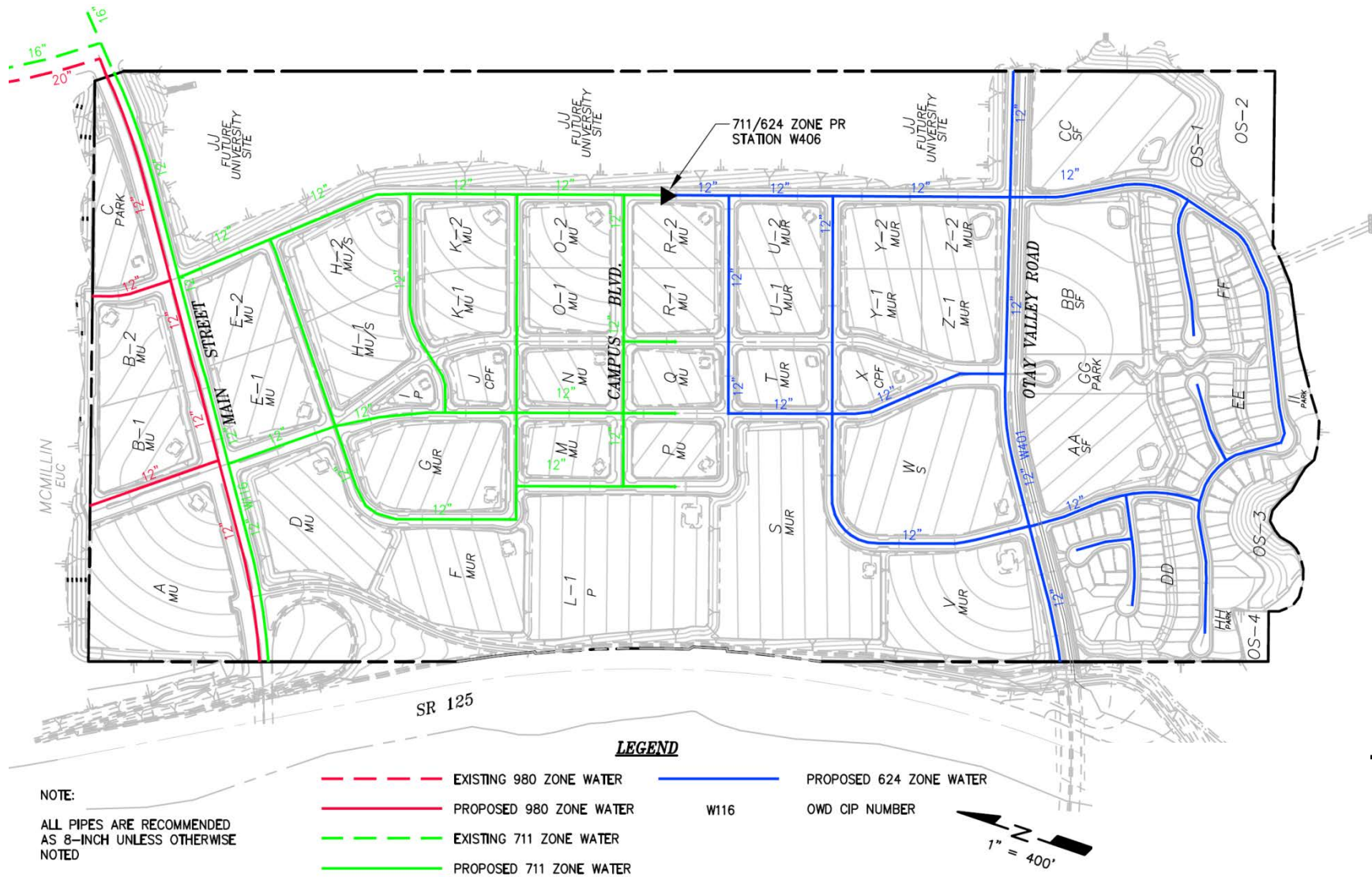
EXHIBIT 4.7.3 ON-SITE POTABLE WATER FACILITIES
