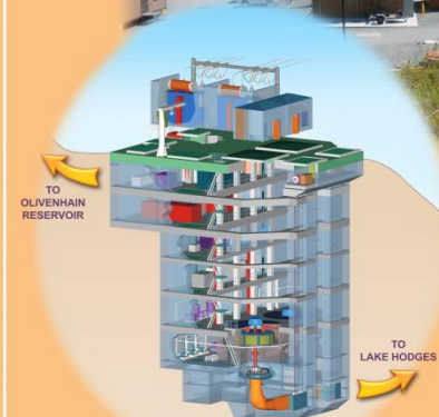
Pump House Detail
