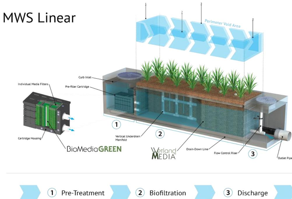
7. Biofiltration BMP must include operations and maintenance design features and planning considerations to provide for continued effectiveness of pollutant and flow control functions.
