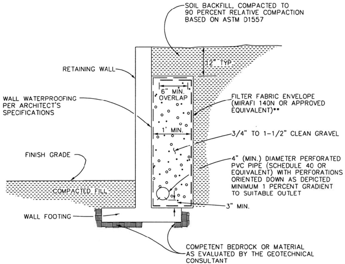
NOTE: UPON REVIEW BY THE GEOTECHNICAL CONSULTANT, COMPOSITE DRAINAGE PRODUCTS SUCH AS MIRADRAIN OR J-DRAIN MAY BE USED AS AN ALTERNATIVE TO GRAVEL OR CLASS 2 PERMEABLE MATERIAL. INSTALLATION SHOULD BE PERFORMED IN ACCORDANCE WITH MANUFACTURER'S SPECIFICATIONS.
