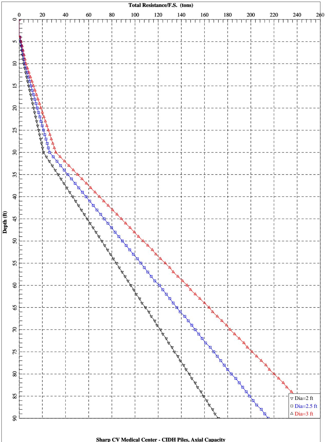
Sharp CV Medical Center - CIDH Piles, Axial Capacity
