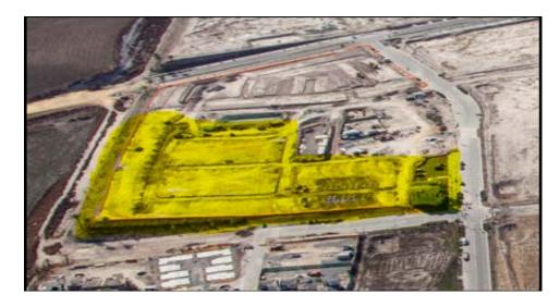
There are two completed models at the northeast corner of the site and six production units are under construction. Most of the grading is complete along with wet utilities. The dry utilities are being installed as the pads get completed. Internal streets have not been paved yet due to the utilities not being finalized.
