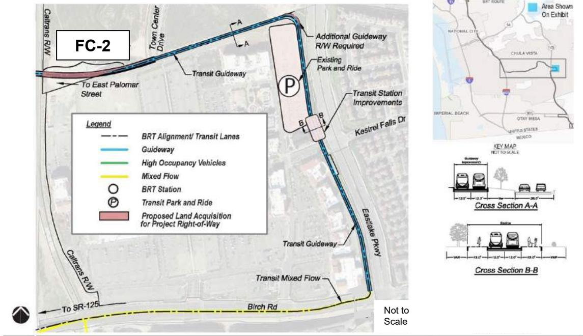
BRT guideway: from the FC-2 site, the guideway crosses over SR-125 via a guideway and pedestrian bridge.
