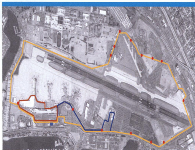
Our campus-wide electrical distribution grid on airport sends solar-generated power where needed.
