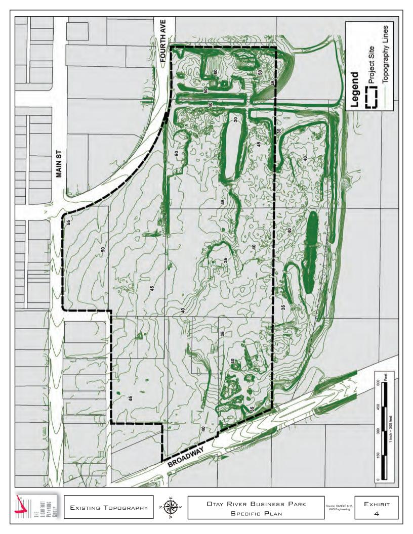
the proposed desilt basin #9. South of Faivre Street, the proposed grading starts at about 50 feet AMSL on the eastern portion adjacent to the future park space and drops to about 45 feet AMSL near the southwest corner of the site, with a slope along the southern boundary of the graded portion of the property.
