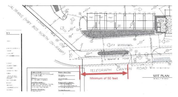
Current plans provided to Caltrans dated September 26, 2017, do not show encroachment in to Caltrans right-of-way. Any work performed within Caltrans right-of-way will require discretionary review and approval by Caltrans and an encroachment permit will be required.
